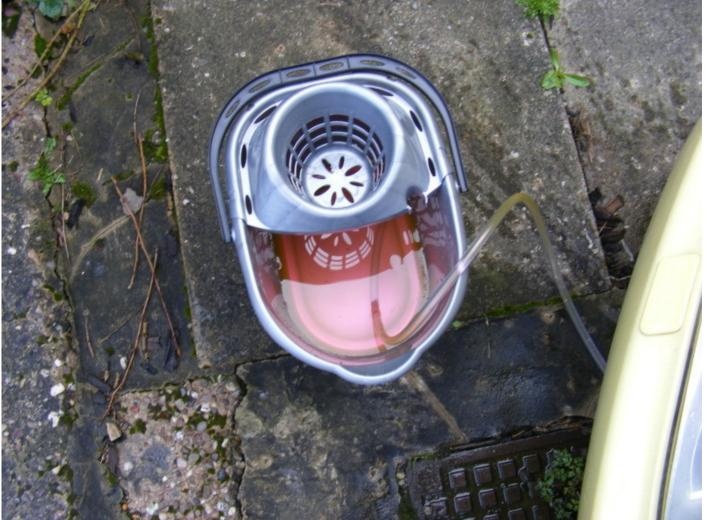
It'll take a few minutes to drain. I made a mistake here & allowed the tube to pick up some dirt & grit, this ended up in the bucket, not a problem though. Once I was done I got another bucket, put a tea towell over it & poured the coolant through it, this acted as a sieve & filtered the dirt out. Do check afterwards though, you may want to sieve it twice.
